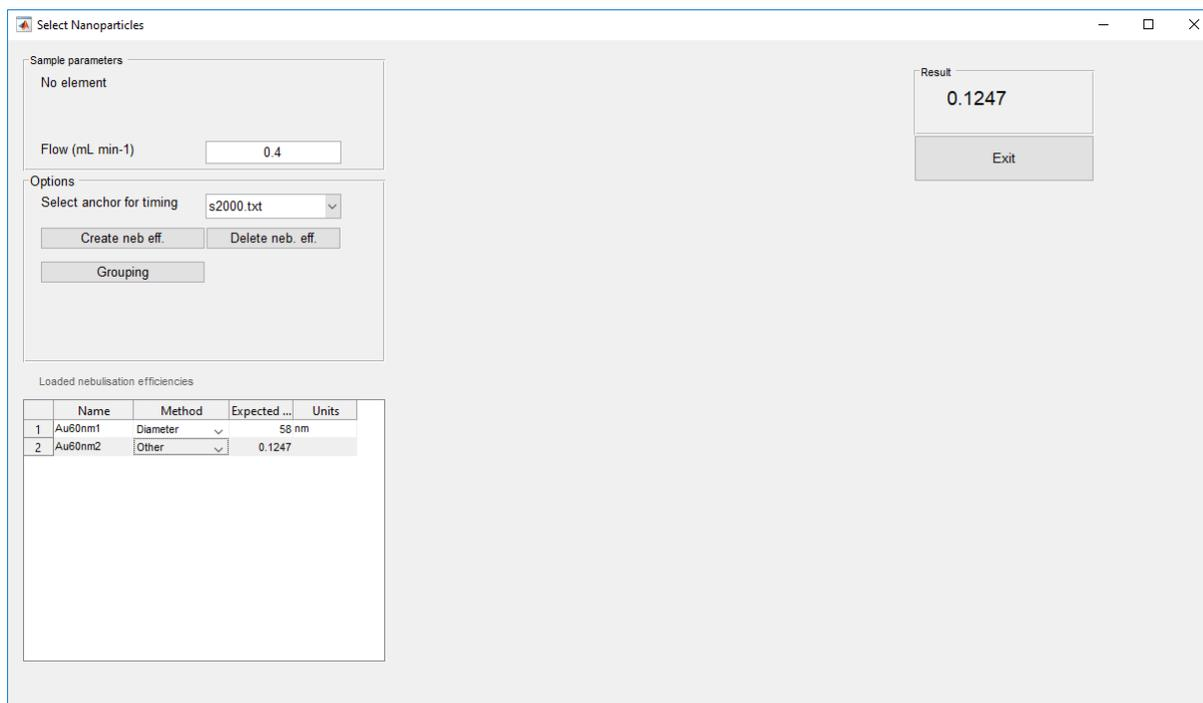
Figure 37 The nebulisation efficiency tool when the “other” method has been chosen
