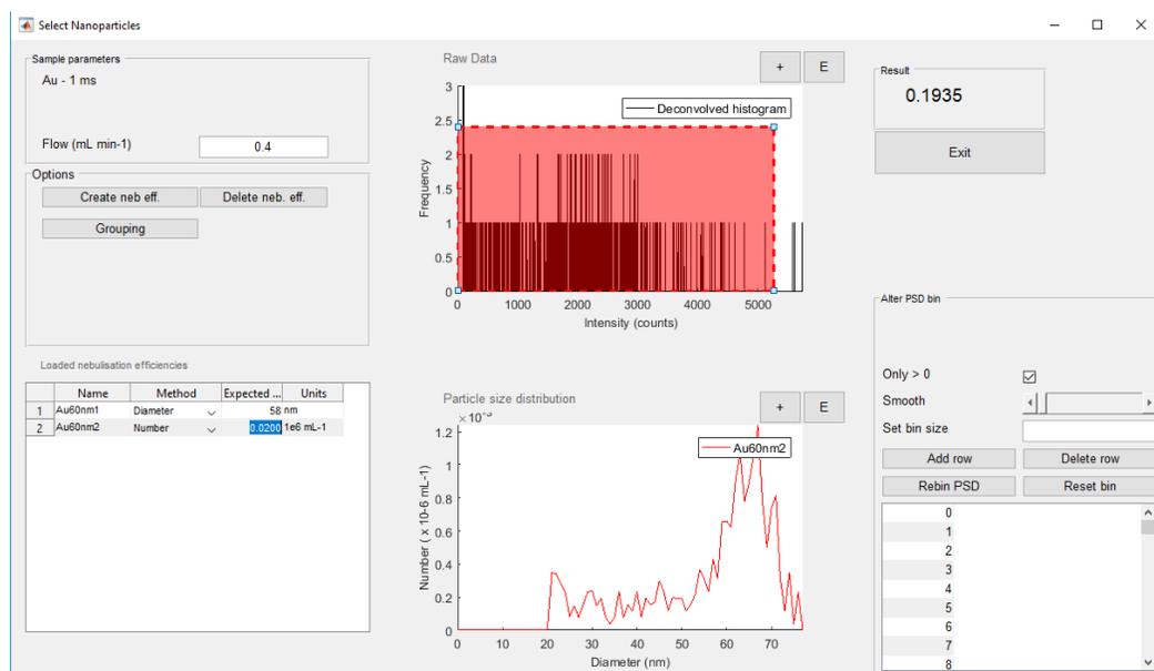
Figure 39. The nebulisation efficiency tool when using the number concentration standard method.
