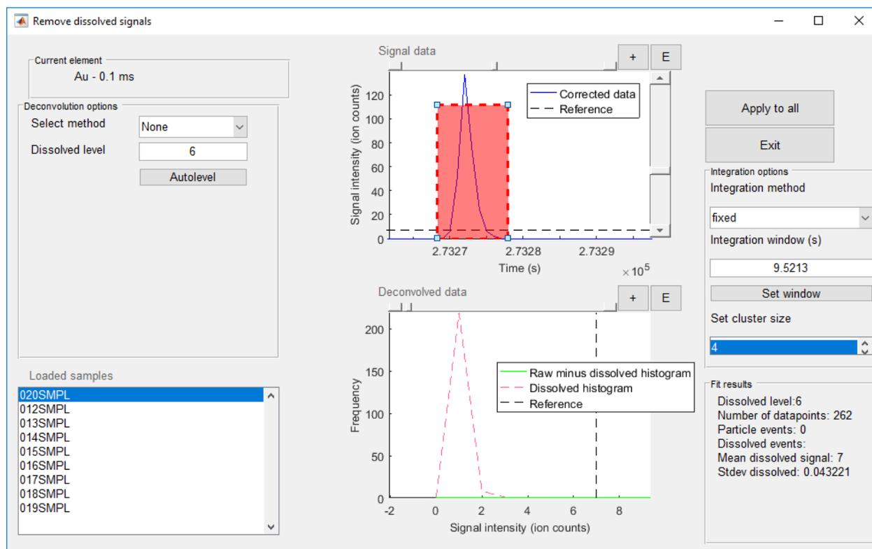
Figure 35. The “remove dissolved signals” tool in the case of a FAST project using the fixed integration method
