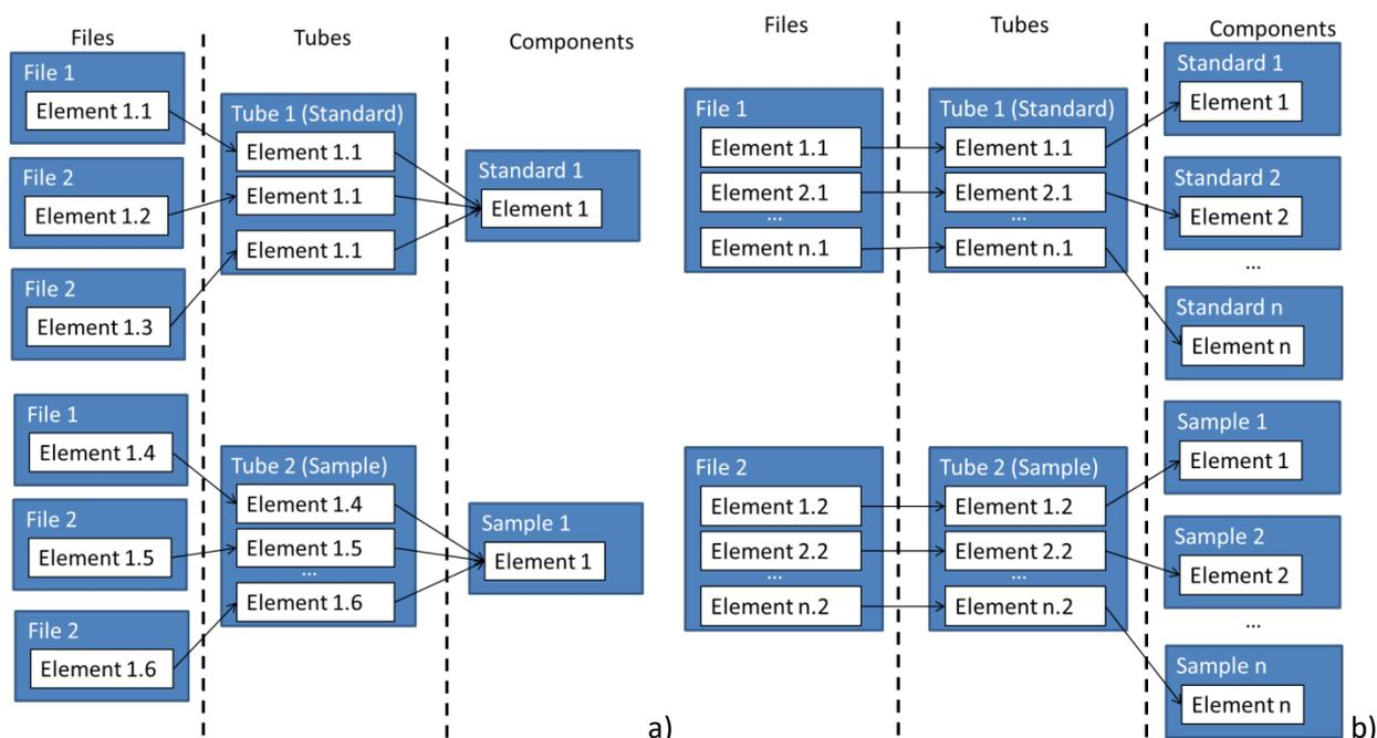
Figure 15 Two typical import sequences for a) a single element case and b) a multi-element case. The first stage is performed in the “import files tool” where files and tubes are linked. The second stage, where tubes are transformed into components is done in the “declare import rules” tool.
