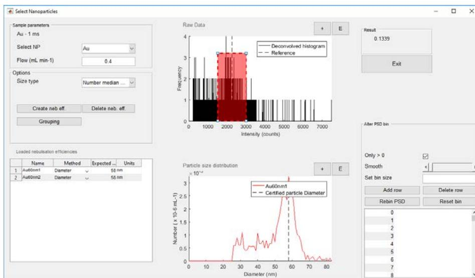
Figure 38 The nebulisation efficiency tool when using the diameter method.
